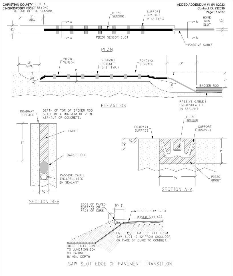
PIEZOELECTRIC SENSOR INSTALLATION
