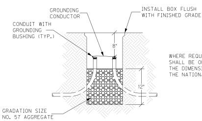
WHERE REQUIRED, JUNCTION BOX SHALL BE ORIENTED SUCH THAT THE DIMENSIONS COMPLY WITH THE NATIONAL ELECTRICAL CODE.
